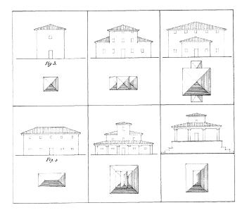
Fig. 2. Classifications of the elements of architecture based on formal typology by J.N.L.Durand. Following Quatremère's typological principles, this was a deliberate attempt to reduce architectural design to composition with pre-determined forms.
